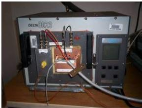
**Delta Design 9023 Environmental Test Chamber**—Allows for precise temperature control within the range of -180°C to 315°C. (208 Rhines)
