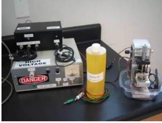
**Ferroelectric Characterization-** The hysteresis curves are extracted from this custom made high voltage source (max 4 kV) and measuring apparatus. (208 Rhines)
