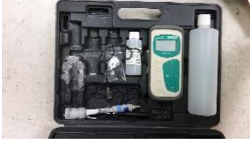
**pH/mV/°C Meter-** Can measure pH, absolute mV, relative mV and temperature. (256 Rhines)
