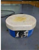
**Fisher Scientific Thermix 120S Small Vessel Stirrer-** This is used for mixing. (Speed: 200-2500 rpm Diameter: 6in Height: 3in) (256 Rhines)
