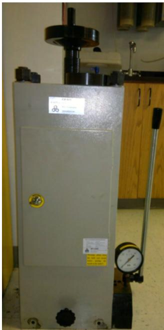
**Isostatic press** – An isostatic press is used to exert a uniform and 3-D force on a sample by applying pressure to an oil chamber containing the sample. This 3-D pressure is useful to achieve a greater sample density as the entire surface area of the sample experiences the resulting compression. This particular isostatic press exerts a maximum of 34 MPa of pressure. Model CIP-50M. MTI Corp. (256 Rhines)
