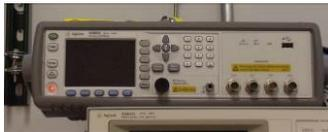
**Precision LCR meter (Agilent E4980A)** –Used to measure inductance, capacitance and resistance of a sample/component. Frequency range of 20 Hz to 2 MHz. (208 Rhines)
