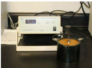
**Piezoelectric Meter-** The PM3500 is manufactured by KCF Technologies and enables  $d_{33}$  and  $d_{31}$  measurements. The 90-2030 model from APC Ceramics Inc. measures a wide-range of 1-2000 pC/N, accommodates various sizes and shapes, and can determine polarity. (208 Rhines)
