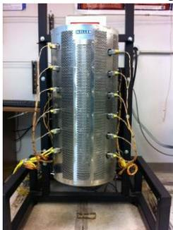
**1300°C EDG Vertical Tube Furnace (bore dimension 3x24 inches)** - from Mellen Company, Inc., is configured with 24 individually controlled heater zones which allows for a precise and dynamic control of the temperature profile. The temperature gradient can be programmed to translate along the length of the furnace bore, which eliminates the need for a dropping motion of the sample during crystal growth. (208 Rhines)
