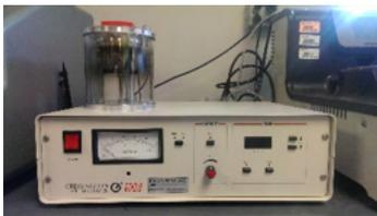
**Sputter Coater-**The sputter coater is used to coat otherwise non-conducting samples for SEM or x-ray scattering analysis. This particular sputter coater is capable of sputtering gold or platinum. (208 Rhines)
