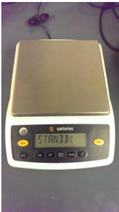
**Sartorius Digital Balance** – The Sartorius Entris digital balance is a larger digital balance with a capacity of 2200g with a readability and precision of 0.01g. The larger pan offers the ability to measure larger amounts of materials and greater flexibility. (256 Rhines)
