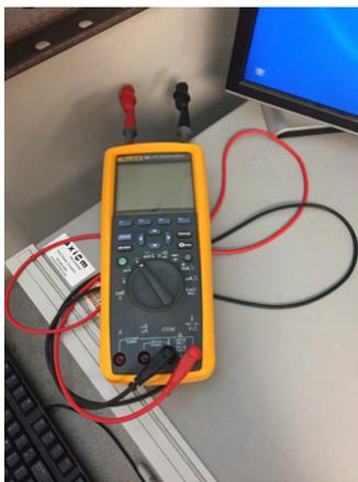
**Fluke 289 True-RMS Industrial Logging Multimeter** – High-performance multimeter capable of measuring AC/DC voltage, AC/DC current, temperature, resistance, capacitance, frequency, connectivity
