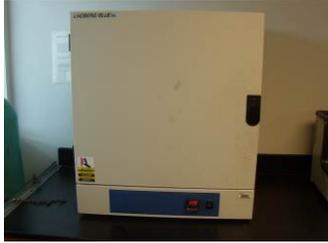
**Drying Oven-**Quincy Labs, Inc. oven (model: 10 GC) and Fisher Scientific, model 650G featuring temperature range of 50-225°C and 5.0 ft<sup>3</sup> capacity. Used to dry a sample before pressing or analysis. (256 Rhines)
