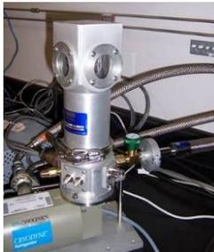
**Cryo-refrigerator -** Temperature from 15 K to 500 K can be achieved, with 4 BNC connectors that can be connected to electrical characterization equipment such as LCR. (208 Rhines)
