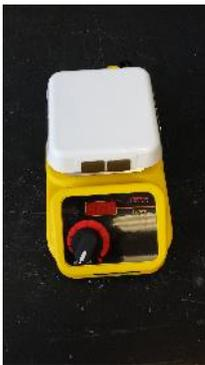
**Thermo Scientific Cimared - Hot plate** - A hotplate is used for baking and curing thin films and coatings. This hot plate allows a temperature resolution of 2°C and a Temperature Range of 5 - 400°C. (256 Rhines)
