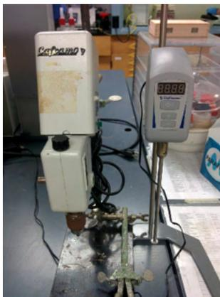
**Caframo Overhead Mixer Stirrer: RZR1(left) and BDC250(right)** – Stirrers for mixing reactions, samples, and solutions.
