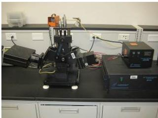
**J.A. Woolam Ellipsometer**—The ellipsometer is able to measure the refractive index and the thickness of semi-transparent thin films. It can be used to measure layers as thin as 1 nm up to layers which are one micron thick. Applications include the accurate thickness measurement of thin films, the identification of materials and thin layers and the characterization of surfaces.
