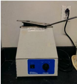
**Sonicator** – Used to agitate and disperse particles within a solution. This is useful in creating a uniform solutions, emulsions, and suspensions in relatively short periods of time. Can also be used for ultrasonic cleaning of equipment as the ultrasound loosens particles adhering to a surface. (256 Rhines)
