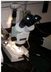
**Optical Microscope** - The Meiji EMZ 13TR Stereo Microscope also includes digital capture and a wide range of magnifications from 60X to 420X. (208 Rhines)
