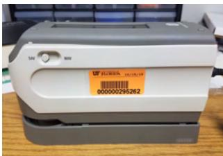
**Konica Minolta CM2600d Photospectrometer** - Used to measure the precise color of a sample using a variety of standardized color coordinate systems. (208 Rhines)
