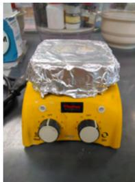
**Thermo Scientific SP194715 Hot Plate-**A hotplate is used for baking and curing thin films and coatings. (Speed: 100-2500 rpm Temperature resolution: 1°C Temperature Range: 150-538°C Voltage: 120V Amp: 3.45A Herz: 60Hz) (256 Rhines)
