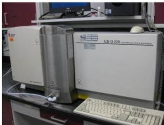
**Coulter LS320- B** measures particle size from 40 nm to 2mm by laser light scattering (LS). This instrument has three sample modules: a Universal Liquid Module, a Micro-Fluid Module and a Dry Powder Module (DPM). Samples in both powder and liquid form can be measured.
