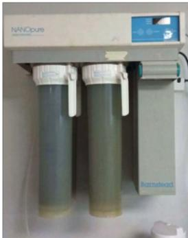
**NANOpure Water purification system** – This is used to purify the water (256 Rhines)
