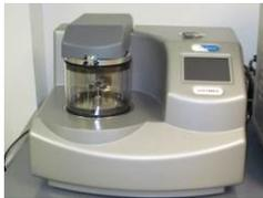
**Carbon Coater-**The carbon coater is used to coat otherwise non-conducting samples for SEM or x-ray scattering analysis. The EMS150R E from Quorum Technologies is a compact rotary-pumped carbon coater. (256 Rhines)
