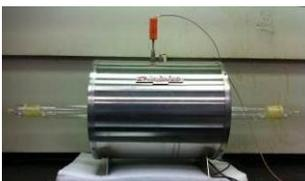
**1200°C Atmosphere Tube furnace** - (chamber dimensions 2x10 inches) – from CM Furnaces Inc., Programmable Ramp and Soak controller. Used for  $\text{BiI}_3$  powder synthesis through physical vapor transport. (208 Rhines)
