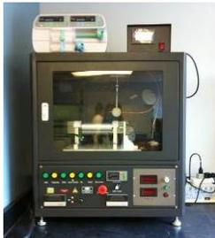
**NaBond Electro-spinning and Spray Unit-**This system uses electrostatic and mechanical force to spin nanofibers with diameter of 20-1000nm from a solution/molten precursor. Single nozzle, multi nozzle, and coaxial nozzle spinnerets available. High voltage power supply reaching 50kV. Many options for rotating collectors are available including drum and disk collectors. (256 Rhines)
