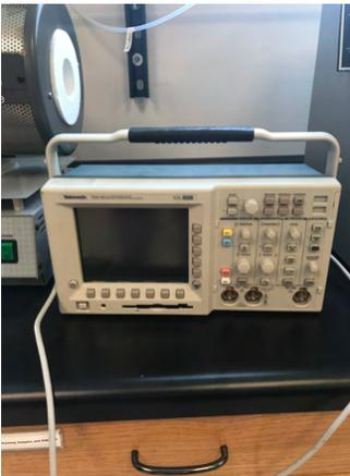
**TDS 3012 Two Channel Color Digital Phosphor Oscilloscope** - from Tektronix. (208 Rhines)
