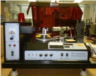
**Single Crystal Orientation Device** – The EQ-DX-100G (MTI Corporation) is a desktop X-Ray diffractometer used for analyzing the orientation of single crystals in a  $2\theta$  range from  $10^\circ$ - $140^\circ$ . (208 Rhines)
