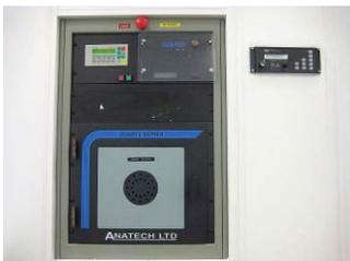
**Anatech Barrel Asher SCE600**-Uses an oxygen plasma for stripping photoresist, descum, surface cleaning, and surface treatment. Can process up to 25, four inch wafers at one time. Max power is 600W.
