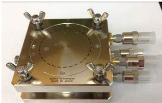
**Agilent 16452A Liquid Test Fixture**—Provides accurate dielectric constant and impedance measurements of liquid materials. The fixture allows you to make frequency swept measurements or temperature coefficient measurements that precisely characterize liquid materials. (208 Rhines)
