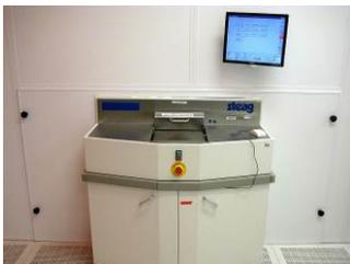
**Steag RTA 100CS RTP**-Atmospheric Rapid thermal anneal to 1050°C. Gases available are: N<sub>2</sub>, H<sub>2</sub>+N<sub>2</sub>, O<sub>2</sub>. Process time is limited to 10 minutes.
