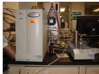
**Quantachrome Porometer 3G-zh** - Measures pore sizes using a liquid expulsion technique. The pore size distribution that the system measures is in the range of 500 $\mu$ m down to 18nm. The pressure used to measure these pore sizes is 500psi.
