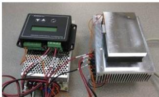
**Peltier-Thermoelectric Cold Plate Cooler -** from TE Technologies, provides effective, direct-contact cooling for small heat loads at low temperatures. The plate temperatures can be cooled down to below -20°C. (208 Rhines)
