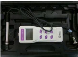
**Fisher Scientific Traceable Expanded Range Conductivity Meter** – Used for checking the purity of water from stills, deionizers, and reverse osmosis, testing laboratory glassware rinsing, measuring total dissolved solids, and making solutions. (256 Rhines)
