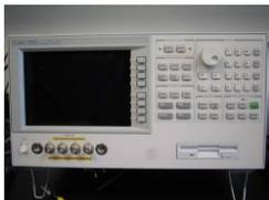
**Precision Impedance Analyzer (Agilent 4294A)** - Frequency range of 40 Hz to 110 MHz. (208 Rhines)
