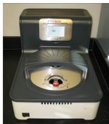
**Planetary Ball Mill**—This ball mill uses uniform balls in a rotating bowl to reduce the size of particles within the mill. The Fritsch Pulverisette 7 has 70 ml zirconia milling bowls that can rotate up to 1100 rpm and can produce a final particle size of <0.1 μm. (256 Rhines)
