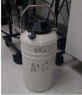
**Nitrogen Dewar - MVE - Lab 5-** Container used for storing of liquid nitrogen. Net capacity is 5 Liters, static evaporation rate is 0.15, neck opening of 2.2 inches, overall height of 18.2 in. (208 Rhines)
