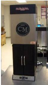
**1800°C Bottom Loading and Quenching Furnace** - (chamber dimensions 6x6x6 inches) – from CM Furnaces Inc., includes a multi-step programmable controller and bottom lowering motor. (208 Rhines)
