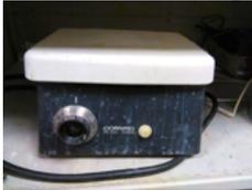
**Corning PC-353 Stirrer-** This is used for mixing. (Speed: 80-1000 rpm measures: 5x7in) (256 Rhines)
