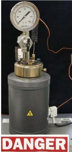
**Pressure Reactor (Autoclave)** - Designed for creating conditions for reactions that require high pressures and temperatures. Used for the growth of crystals from a variety of solvents at different concentrations. (208 Rhines)
