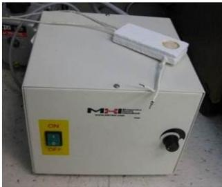
**HeatPad™ Microheater -**Rapid heated area (1 inch size) up to 1200°C (measured at internal thermocouple). Low heater profile enables localized heating, substrate heating, vacuum environments and high pressure environments. (208 Rhines)
