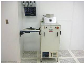
**PECVD, STS 310PC**-The PECVD STS deposition tool is used for depositing silicon nitride, silicon dioxide and amorphous silicon films. The system is equipped with 13.56 MHz and 187.5 kHz frequencies and is capable of mixed frequency recipes. The temperature of the system is normally kept at 300 °C.
