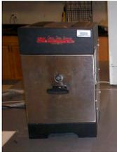
**1700°C Rapid Heating furnaces (2)**- (chamber dimensions 4x4x4 and 8x8x8 inches) – from CM Furnaces Inc with multi-step programmable controller and optical window. (208 Rhines)
