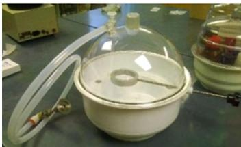
**Vacuum Chamber** – Used in PIP (polymer impregnation and pyrolysis). It is specifically used to supplant air in pores of a sample with polymer. The tube is connected to a roughing pump and the arm holds a 100 mL beaker which is used to pour the polymer onto the sample(s). (256 Rhines)
