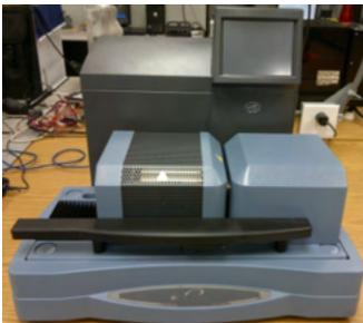
**Simultaneous TGA/DSC** – The SDT Q600 provides simultaneous measurement of weight change (TGA) and true differential heat flow (DSC) on the same sample from ambient to  $1500^\circ\text{C}$  in air or gas-controlled atmosphere. (208 Rhines)
