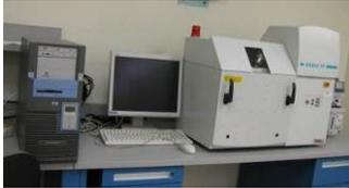
**EDAX Inc. Micro-XRF Elemental Analyzers** -A compact, tabletop instrument used for elemental analysis based on X-ray fluorescence (XRF). It features fast, simultaneous, non-destructive sample analysis with little or no sample preparation for most materials. (125 NSC)
