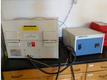
**Tube furnace and Controller** - Lindberg blue furnace (Model number: HTF55322A Chamber diameter: 1-3 inch) works within a temperature range of 100°C - 1200°C. (208 Rhines)
