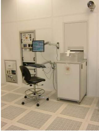
**STS Deep RIE**—Used to modify the physical properties of a target using a plasma. This process is essential in the fabrication of integrated circuits. The STS DRIE is an Inductively Coupled Plasma Process etcher designed and configured to etch deep high aspect ratio features in silicon only. The process provides high selectivity for etching Si with most common Photoresist and SiO<sub>2</sub> masks.
