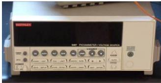
**Keithley Picoammeter (6487)** - Measures currents ranging from 20fA to 20mA, takes up to 1000 readings per second, and source voltage from 200μV to 505V. (208 Rhines)
