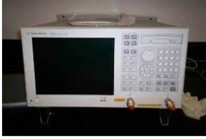
**Agilent Technologies E5071B-** A network analyzer measures RF components within the frequency range of 300 kHz - 8.5 GHz. (208 Rhines)
