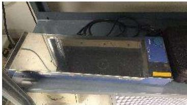
**IKA RO 10 Power IKAMAG Magnetic Stirrer-** Multi-position magnetic stirrer with 10 stirring positions, without heating. The stainless steel surface covers the unit allowing easy cleaning and providing protection against the penetration of liquids. (256 Rhines)
