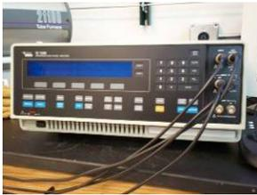
**SI 1260-** A Solartron impedance/gain-phase analyzer. Frequency range from 0.1 Hz to 32 MHz. (208 Rhines)
