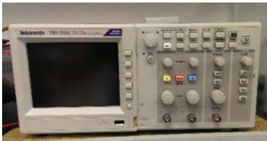
**Tektronix TBS1022 2 Channel Oscilloscope** – This instrument is used to observe the change of an electric signal over time. This model is a 2 channel oscilloscope with a 500 MS/s sample rate and a 8 bit vertical resolution. (208 Rhines)
