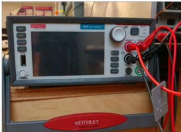
**Keithley Model 2450 SourceMeter** - benchtop Source Measure Unit (SMU) instrument. Acts as power supply, current source, DMM, electronic load, and trigger controller. (208 Rhines)
