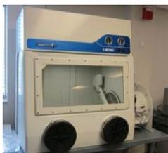
**Glove Box** – The glove box is used for precise control of the atmosphere, or lack thereof, in which a sample is being worked on. This glove box model 5220100 from Labconco provides a leak-tight environment for work with contamination-sensitive materials. (256 Rhines)
