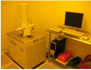
**JEOL 5700 Electron Microscope**-The JEOL CarryScope is a compact and portable SEM that utilizes a standard tungsten filament. The CarryScope is capable of imaging from 8X to 300,000X and up to 5nm resolution. Accelerating voltage can be varied from 5kV to 20kV and the beam diameter can also be adjusted. It features manual XYZ stages with full 360° rotation and -10° to 90° tilt and can hold a full 4" wafer.
