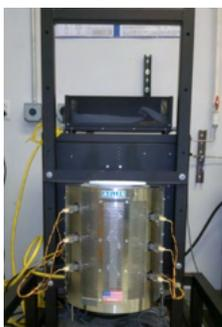
**1300°C EDG Vertical Tube Furnace (bore dimension 3x24 inches)** - from Mellen Company, Inc., is configured with 12 individually controlled heater zones which allows for a precise and dynamic control of the temperature profile. The temperature gradient can be programmed to translate along the length of the furnace bore, which eliminates the need for a dropping motion of the sample during crystal growth. (208 Rhines)
