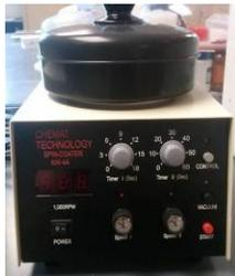
**Chemat Scientific KW-4A Spin Coater**– A spin coater deposits a film/coat by using a two-stage spin process which includes dispensing the film/coat at low speed and homogenizing the film/coat at high speed. The KW-4A spin coater can be used to deposit metal oxide thin films, polymer coatings and metal organic thin films. Stage 1 rotation speed 500-2500rpm, Stage 2 rotation speed 800-8,000 rpm. (256 Rhines)
