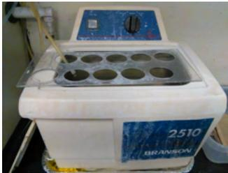
**Branson 2510 Ultrasonic Cleaner** – Tank Size: 6" x 5.5" x 4"(LxWxD) Tank Capacity: 1/2 gallon Frequency: 40 kHz (208 Rhines)
