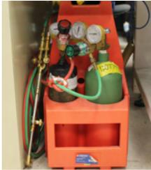
**Campbell Hausfeld WT500000AV Porta-Torch Kit** – Used to heat and weld something. It has gas cylinder of oxygen (right) and acetylene (left). (208 Rhines)
