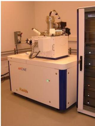
**Raith ionLINE- multi-species FIB**-The Raith ionLINE is a focused ion beam (FIB) lithography system with a Liquid Metal Alloy Ion Source (LMAIS) rather than traditional Ga for exposure, milling, and implantation.
