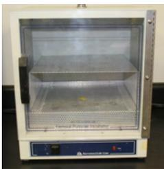
**Incubator** - Barnstead international (model: 150), operating temperature ambient to 40°C, with the chamber dimensions (12.7" W x 13.4" L x 12.7" H). (208 Rhines)
