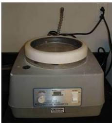
**Model 900 Grinding and Polishing Machine** -from Southbay technology. The grinding machine is used to polish a ceramic pellet by using progressively finer polishing pads to smooth the sample's surface. (256 Rhines)
