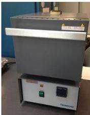
**Thermo Scientific Benchtop Muffle Furnace (2)**-Excellent for quantitative analysis, quenching, and organic and inorganic ashing applications. The furnace can run up to 1200°C and has high thermal-shock resistance. (208 Rhines)
