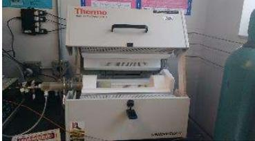
**Custom Made Quartz Reactor -** Design allows the maintenance of different atmospheres (partial pressures of hydrogen) on the opposite sides of the sample required for proton transference number measurement. A thermocouple located close to the sample minimizes error in temperature measurement. The reactor is also used for variable atmosphere conductivity measurement as a function of temperature. (208 Rhines)
