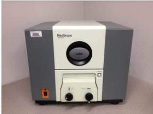
**JOEL NeoScopeBenchtop SEM** –Scanning electron microscope with magnification is from X10 to X40,000. It has accelerating voltages of 15 kV, 10 kV, and 5 kV in a 3-position switch. High and low vacuum modes. Secondary electron and backscattered electron imaging. Sample loading to imaging in less than three minutes. (208Rhines)
