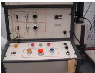
**Quantachrome Autoscan 60 Mercury Porosimeter** - Measures open pore size distribution with pore radii varying from ~100  $\mu$ m to 1.8 nm for unconsolidated and consolidated particulate materials. Mercury is used at high pressure to determine the pore size.
