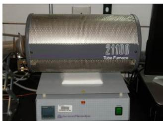
**SType F2110 Tube Furnace** - A Barnstead International furnace works within a temperature range of 100°C - 1100°C. Used for high temperature electrical measurements. (208 Rhines)
