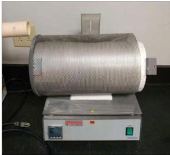
**Lindberg Tube Furnace (2)** – Model Number: F21135 Tube Furnace, multi-position, heats from 100°C to 1200°C. (Rhines 208)
