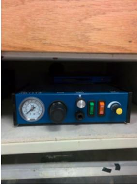
**I&J Fisnar Liquid Dispenser** – Analog pneumatic liquid dispenser that can be used as a syringe pump. Suitable for all types of fluids. Barrel suck-back ensures no dripping. Air input 70 to 100 psi, air output 1-100 psi. (256 Rhines)
