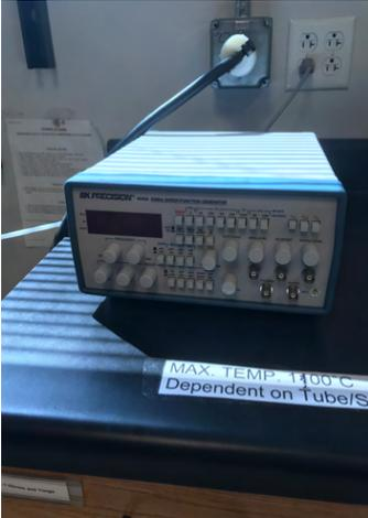
**20MHz Sweep/Function Generator** – from BK Precision, model: 4040A, allows for sine, square, pulse, and ramp output. (208 Rhines)
