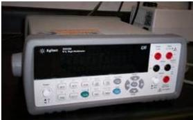
**Digital Multi-Meter (2)-** The Agilent 34401A has a 6.5 digit display and can be used to measure DC/AC voltage, DC/AC current, 2 and 4 wire resistance, diode, continuity, frequency and period. (208 Rhines)
