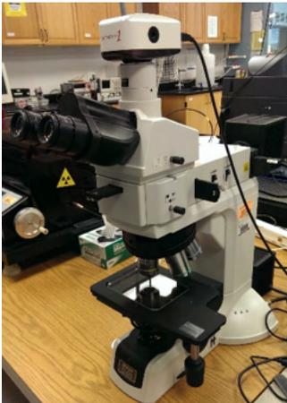
**Nikon Eclipse LV100-** A polarizing optical microscope with 5 objectives ranging from 4x to 100x giving a magnification of up to 1000x. (208 Rhines)
