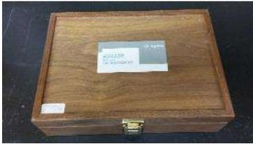
**Agilent 85033E Calibration Kit-** The Agilent 85033E calibration kit contains precision 3.5mm standards used to calibrate Agilent network analyzers. Standards include fixed terminations, open circuits, and short circuits in both sexes. A torque wrench is also included for proper connection. This kit is specified from dc to 9 GHz. (208 Rhines)
