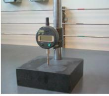
**Digital Comparator** - Mitutoyo thickness meter with an accuracy of  $\pm 0.001$ mm. (256 Rhines)
