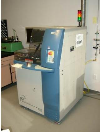
**ADT Dicing Saws**-Fully automatic programmable dicing saw.
