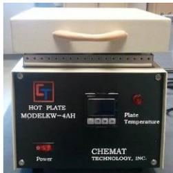
**Chemat Scientific KW-4AH Hot Plate**-A hotplate is used for baking and curing thin films and coatings. The KW-4A hot plate allows a temperature resolution of 1°C and a Temperature Range of 50-350°C.(256 Rhines)
