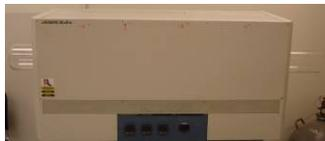
**1100°C 3-zone Tube Furnace** - from Lindberg/Blue M (bore size 6", tube length 60") with multi-step programmable controller and gas/atmosphere flow intake and exhaust. (125 NSC)
