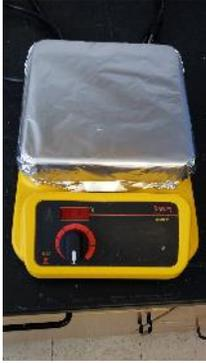
**Thermo Scientific Cimarec - Hot plate** - A hotplate is used for baking and curing thin films and coatings. This hot plate allows a temperature resolution of 2°C and a Temperature Range of 5 - 400°C (256 Rhines)
