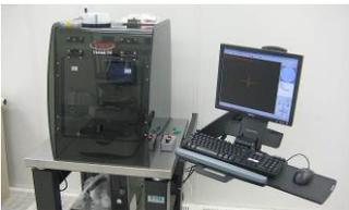
**Profilometer** - The Dektak 150 is a stylus profilometer which can measure step heights and surface roughness by measuring deflections of the diamond-tipped stylus as it is dragged across a surface.
