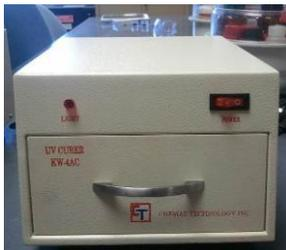
**Chemat Scientific KW-4AC UV Curer**- The KW-4AUV is specially designed for curing photosensitive coatings and thin films. It uses two UV light sources with radiations at 365 nm and 245 nm.(256 Rhines)
