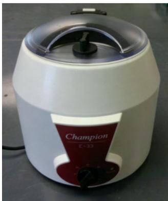
**Centrifuge** – The centrifuge is used to separate particulates out of a liquid in order to isolate a solid or separate a liquid into layers of density. This Champion bench top centrifuge is a single-speed 3300 rpm model with the capacity to hold up to eight 15 mL sample containers. (256 Rhines)
