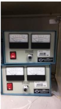
**Voltage Source (2)** Regulated High Voltage DC Power source. (256 Rhines)
