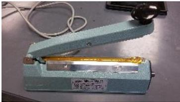
**Manual Sealer-** Impulse Sealer model AIE-200. Used to seal plastic bags. (256 Rhines)
