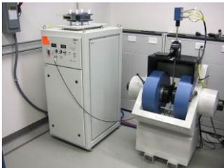
**Lakeshore 7507 Electronic Measurement**—The Lakeshore Hall Measurement System capabilities include Hall coefficient, Hall voltage, resistance, resistivity, magnetoresistance, I-V curves, carrier concentration and mobility.
