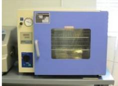
**Vacuum Drying Oven-** This vacuum drying oven model VO-16050 is from Across International. Maximum temperature 300°C, minimum vacuum 0.09 MPa. Used to dry a sample before pressing or analysis when a vacuum is required. (256 Rhines)
