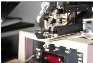
**K&S 4124 Ball Bonder**-Used to make an electrical interconnection between a chip and a device. Used as a part of semiconductor device fabrication. The K & S Model 4124 gold wire ball bonder has the capability of wiring dies to packages or PCBs in a precise and regular pattern. It is stocked with fine pitch capillaries and one Mil pure gold wire.
