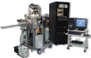
**Sputter Deposition, KJL CMS-18 Multi-Source** - Combinatorial Materials Science thin film sputtering system. 4 gas injected Magnetron sputter sources.
