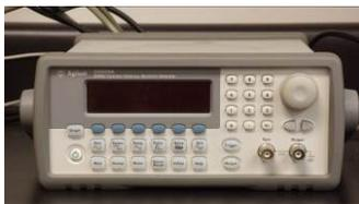
**Agilent 33220A-** A function/arbitrary waveform generator (with AM, FM, PM, FSK, and PWM) modulation types create frequencies within a range of 20 MHz–1  $\mu$ Hz. (208 Rhines)
