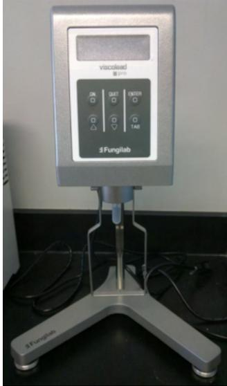
**Fungilab Viscolead Pro Viscometer R** –Measures relative and absolute viscosity, small sample adapter measures 8-13 mL volume solution. Direct readout; Speed: 0.01-200 rpm, Range:100-40,000,000 cP. (256 Rhines)
