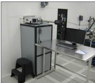
**Cambridge Nano Fiji 200 ALD-A**-A loadlocked ALD system with thermal and plasma deposition capabilities, 3 metal-organic precursors and up to 8" wafer sample size. The system is capable of operating in "exposure mode" which allows for deposition in high aspect ratio features.
