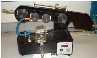
**Bench Top Wire Saw** - from MTI Corporation, model SXJ-2. The bench top wire saw is used to section ceramic samples. This wire saw has a built-in digital micrometer head allowing for 2" travel distance and 0.003 mm accuracy, 360 degree rotating and 30 degree tilt stage, wire traveling speed is 0 – 5 mm/sec, and cutting thickness up to 50 mm. (270 Rhines)
