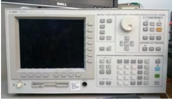
**Precision Semiconductor Parameter Analyzer Agilent 4156C**
