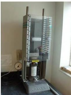
**Hydraulic Press(2)** - Manufactured by Carver (model: 3912) is used in conjunction with die to compress a loose ceramic powder into a pellet using uniaxial force. The clamping force of this particular model is 12 tons. (256 Rhines)
