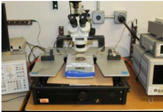
**Benchtop Microprobe Station-** from Micromanipulator (450 PM Test Station) CO., Inc. is a manual analytical probing test station which allows the probing of very small semiconductor geometries. It is available with and 8" chuck and 8 inch by 8 inch stage translation. (208 Rhines)
