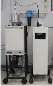
**Anter Flashline 4010 Thermal Properties Analyzer** -Used to determine thermal diffusivity, thermal conductivity and specific heat capacity. Furnace operation from RT to 1600°C with carousel for four (up to 16 mm diameter) specimens in vacuum, air, or inert gas purge. Ranges: Thermal diffusivity: 0.001 to 10 cm<sup>2</sup>/s, Thermal conductivity: 0.1 to 2000 W/mK. (208 Rhines)
