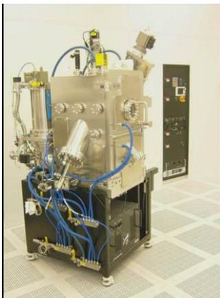
**PVD E-beam evaporator** – Used to deposit layers of atoms on the surface of a sample using a beam of electrons to evaporate the source material and coat all things within a vacuum chamber (sample included). This particular PVD has a 4 pocket 15cc e-beam, a 3” DC sputter source, and a substate heater
