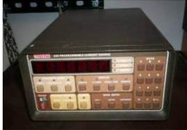
**Programmable Current Source-** A Keithley current source with a full range current from 2 nA to 100 mA and selectable voltage compliance of up to 105 V (in 1 V increments). (208 Rhines)
