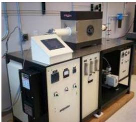
**1800°C Atmosphere/Vacuum Tube furnace** - (chamber dimensions 3x12 inches) - from CM Furnaces Inc., is has an atmosphere controller and multi-step programmable temperature controller. The furnace can also run on vacuum. (208 Rhines)
