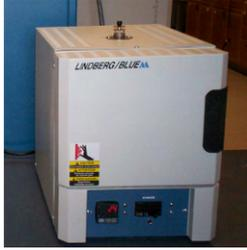
**1100°C Box Furnaces (3)** - from Lindberg/Blue M (interior dimensions 4x8x4, 6x9x6, and 12x18x12 inches) with multi-step programmable controller and gas/atmosphere flow intake and exhaust valves. (208 Rhines)
